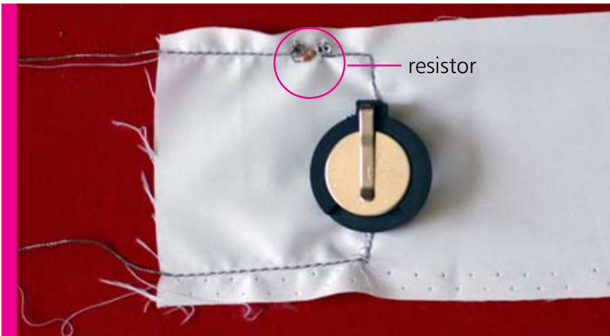
CONNECTING THE BATTERY AND RESISTOR
